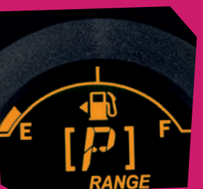
iii. Blinking Low Fuel Level Warning Light
